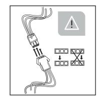
Connector from terminal block to controller.
