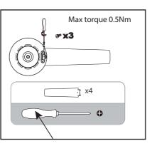
B. Assemble the cover plate to the motor housing with 2 x screws provided. Max. torque to 0.5 Nm.
